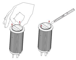
Remove the actuator: lift up the actuator by finger or fine tool toward the edge of the actuator.
